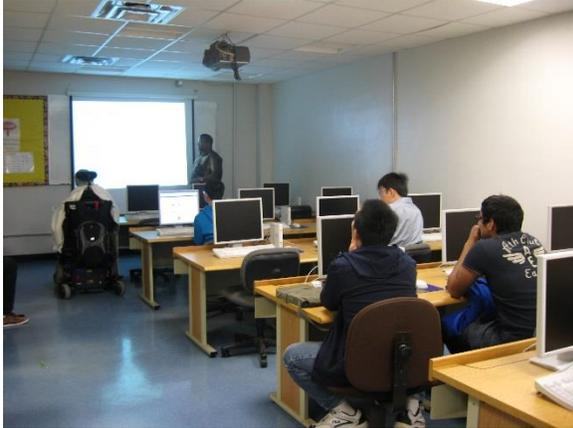
This laboratory consists of new twenty-six (26) Sun Ray clients which are ideal for displaying server-hosted virtual desktops. The desktops in this laboratory are networked and have internet access by way of two (2) Dell PowerConnect 2024 switches.
