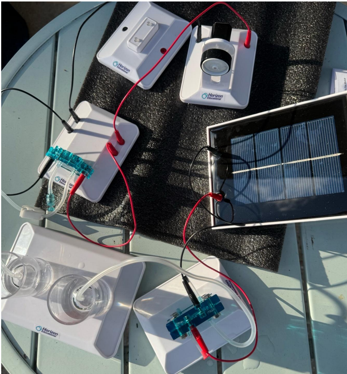
Figure 5: Hydrogen fuel cell powering wheel module
