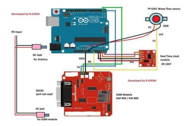
Step 1. With wires connect Arduino pin TX to RX pin in the GSM module.
